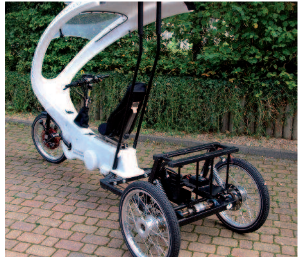
Exposed Chassis shows rear coil springs & battery store
